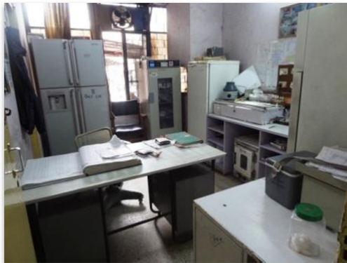
Figure 23: Unrestrained furniture and equipment susceptible to toppling and sliding
