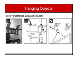
Use hooks to hang pictures, rather than nails so that they do not slide off easily, cause injuries and scatter broken glass.
