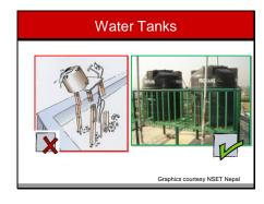
In the Gujarat earthquake many smaller houses were damaged by water tanks from higher buildings toppling over. Position water tanks away from the side with a high enough parapet or railings to prevent it from sliding off the roof. This will also ensure that there is enough water storage available in the tank.
