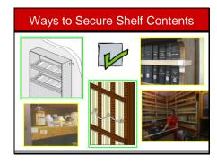
Shelves should be fastened, and the contents of these shelves should be kept from falling. Simple materials can be used to secure shelf contents.
